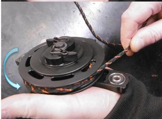
Hold the pulley in place and wind 3 turns of rope counterclockwise.
