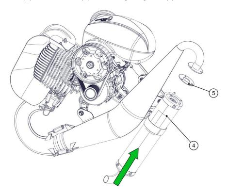
Connect the silencer (4) to the exhaust pipe, inserting the gasket (5).
