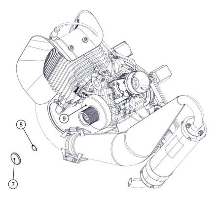
Degrease the seat of the cover on the clutch bell. Insert the cover (7) into the clutch bell (9).
