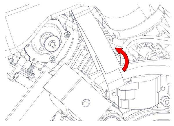
Loosen the screw of the clamp securing the sleeve to the carburettor and remove the airbox.
