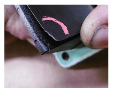
Also check that the petals are not deformed: looking at the inside of the reed valve, the petals should close the opening perfectly (photo on the left). In the photo on the right, you can see deformed petals that remain slightly raised.
