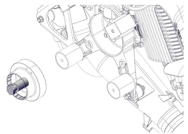
Remove the 2 Allen screws M5x20 (1) with washers (2) from the coil (3). Remove the coil (3).
