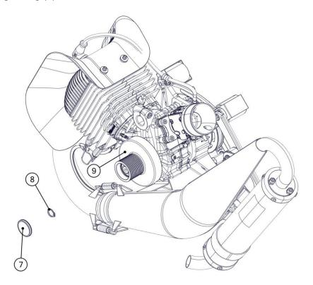
Use an extractor with a maximum hook length of 4 mm.
