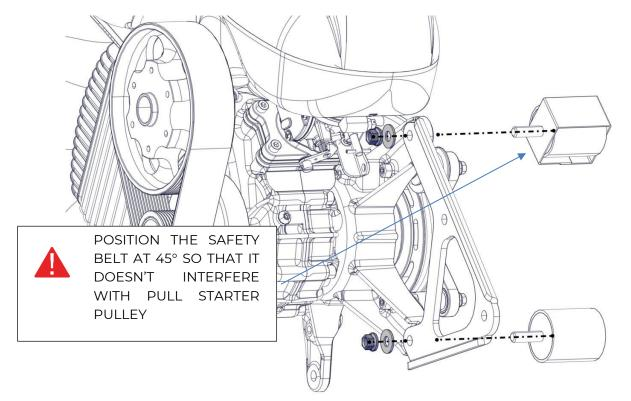
Insert the 2 engine rubber mountings and the 2 self-locking nuts M8 with washers and tighten to 18 Nm.
