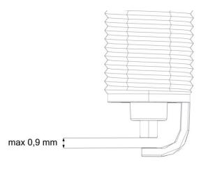
If the distance between the electrodes is equal to or greater than the indicated limit or if scheduled maintenance is required, replace the spark plug.
