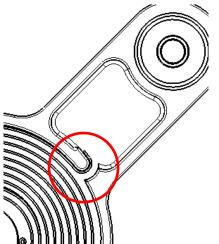
Insert the spring of the hooks on the central pin and turn it, if any blockage or jamming occurs the pin and structure must be replaced.
