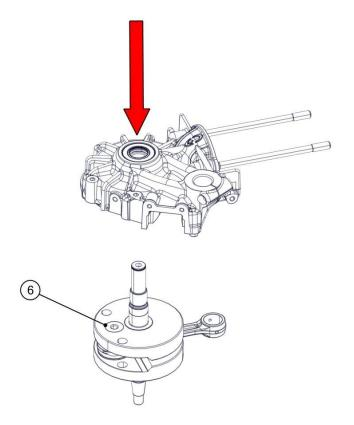
Heat the transmission side crankcase to 120 °C. Remove the bearing (11) and the oil seal (12).
