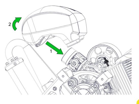
The airbox sleeve (1) must be completely inserted into the Airbox connector (2), the fixing clamp (3) correctly inserted on the seat and aligned as in the figure.
