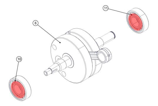
Heat the transmission side crankcase to 120 °C. Insert the crankshaft (6) with the bearings.
