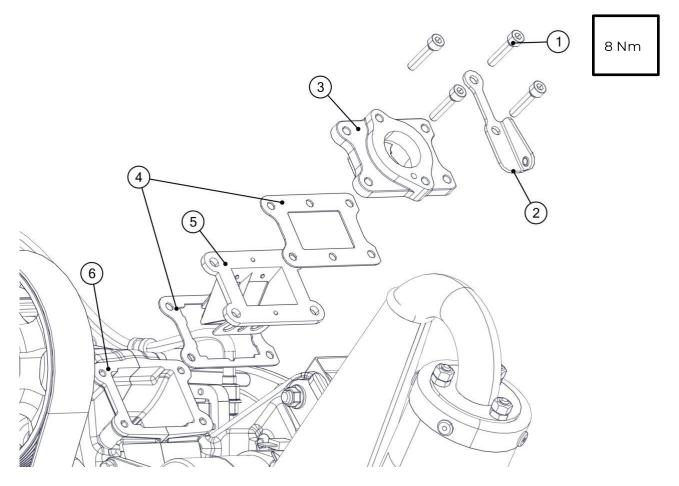
Always replace the gaskets when removing components in contact with them or in the event of leakage. Also, if the motor is not used for a long period of time, check the condition of the gaskets.
