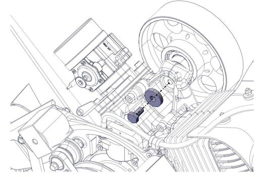
Add Wurth paste 0893921502 to the screw M6x35. Insert the Allen screw M6x35 on the side of the eccentric.
