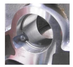
The triangle on the top of the piston indicates the exhaust side.
