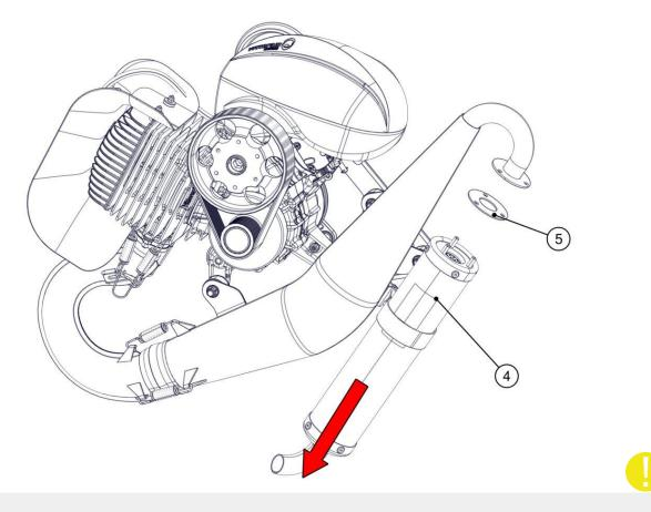
Before disassembling de silencer mark the position of the end caps with a erasable marker
