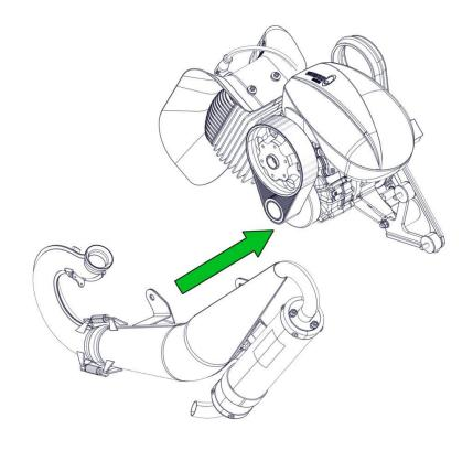
Replace the 3 self-locking nuts M8.
