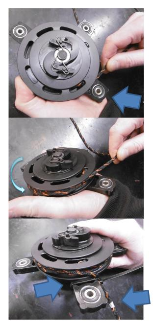
Turn the pulley until you find the origin of the spring tension.
