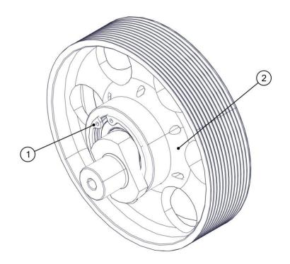
Heat the central part of the pulley to 120 °C. Remove the eccentric (3) with the 2 bearings from the pulley (2).
