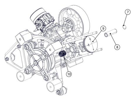
Insert the roller bearing (10), the piston (9), the pin (8) and the circle clip (7).
