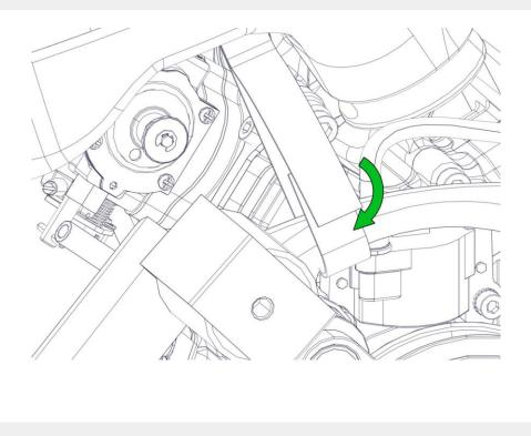
After installation, check that there is no relative movement between the rubber sleeve and the Airbox connector.
