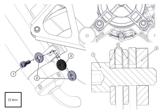
Insert the rubber (3), the 2 washers (2) and the Allen screw M8x25 (1) with threadlocker (recommended Loxeal 83-55/Loctite 270) and tighten to 13 Nm.
