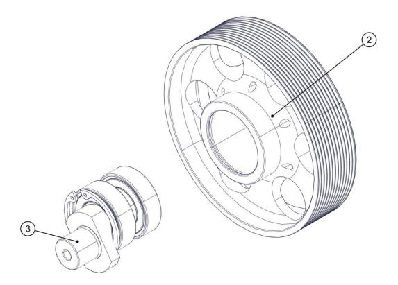
Remove the 2 Seeger rings (1, 4), the 2 bearings (5) with a bearing extractor and the spacer (6) from the eccentric (3).
