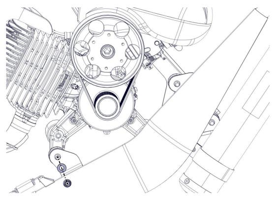
Insert the 2 self-locking nuts M8 with washers on the rubber mountings shown in the figure and tighten to 15 Nm.
