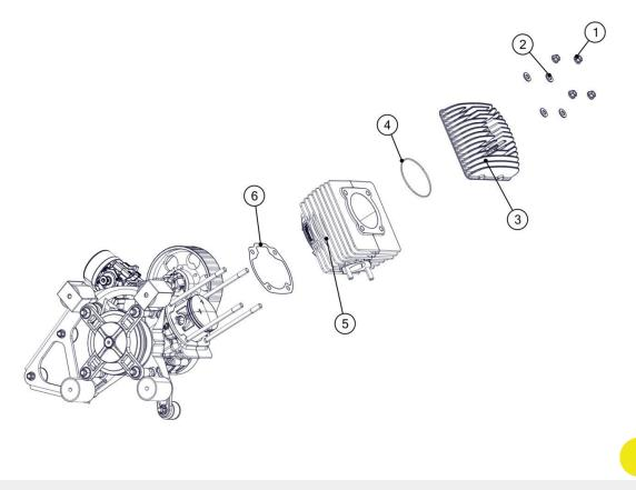
Close the inside of the crankcase with paper to prevent foreign bodies from accidentally falling into the engine.
