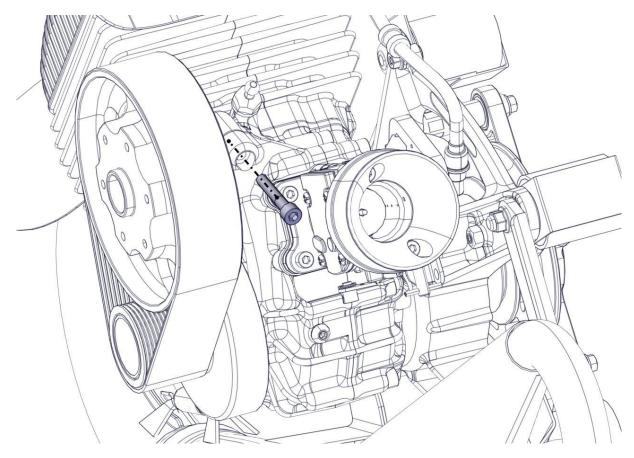
Loosen the hexagonal screw M8x16 on the eccentric.
