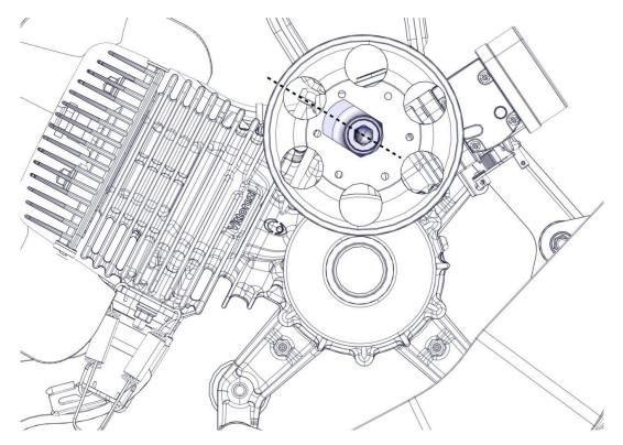
Place the belt on the pulley and clutch bell.
