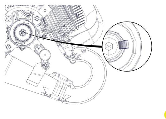
Replace the nut M10x1,25 and the washer 10,5x18.
