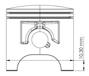
Measure the diameter of the cylinder 10 mm from the top.
