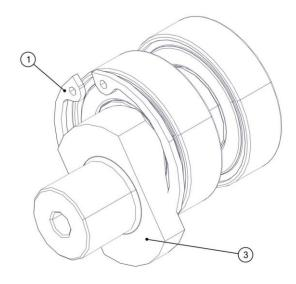
Heat the central part of the pulley to 120 °C. Insert the eccentric (3) with the 2 bearings in the pulley (2).
