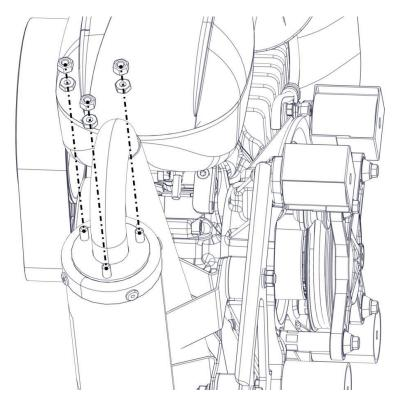
Disconnect the silencer (4) from the exhaust pipe and remove the gasket (5).
