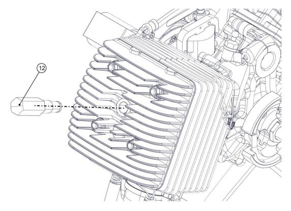
Turn the crankshaft anti-clockwise until the piston is in contact with the piston lock.
