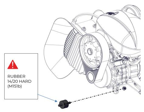
Insert the rubber mounting of the exhaust system shown in the figure, the self-locking nut M8 and tighten to 18 Nm.
