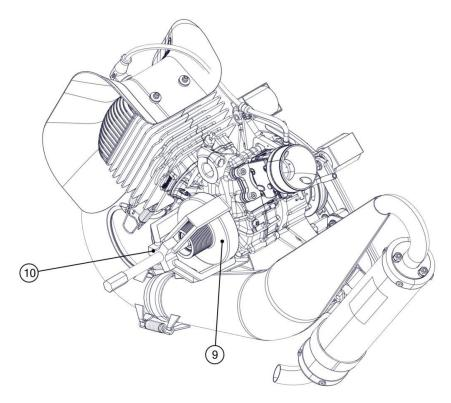
Turn the central pin (11) until the clutch bell (9) is removed.
