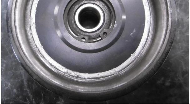
Check the 3 bearing seats: there must be no polished areas. Also measure the diameter of the 3 seats and the internal diameter of the clutch bell, the table shows the factory settings.
