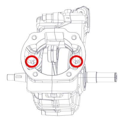
Check the sliding of crankshaft on the bearings.
