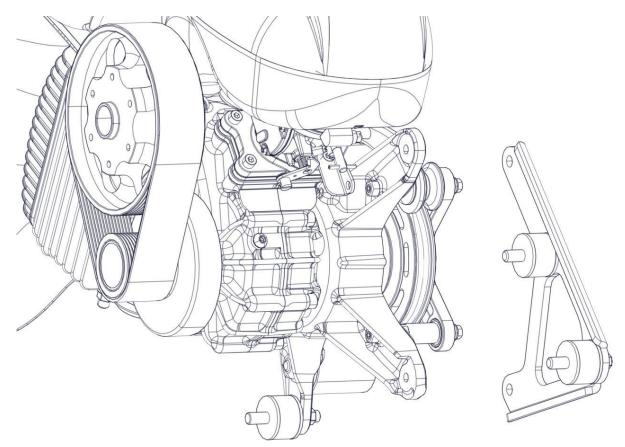
Remove the 2 remaining engine rubber mountings.
