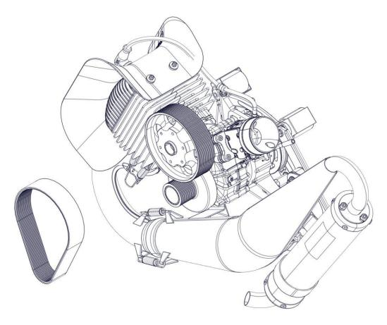
Insert the hexagonal screw M8x16 with washer into the eccentric of the pulley.
