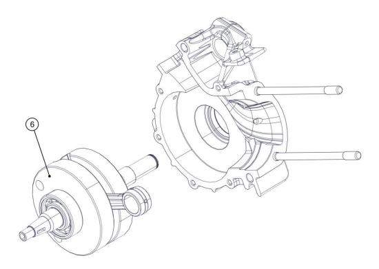
Carry out subsequent operations within a maximum of 5 minutes (application of silicone and closing of the crankcase).
