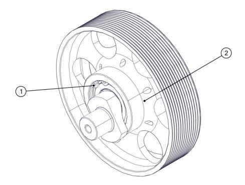
Replace the washer (18) with the same thickness as the ones replaced. Possible sizes range from 0 mm (no washer) to 0,6 mm.
