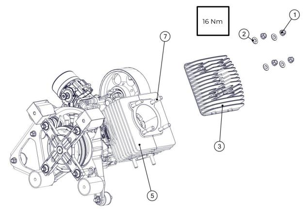
Tighten the nuts progressively, then cross-tighten with the torque shown in the figure.
