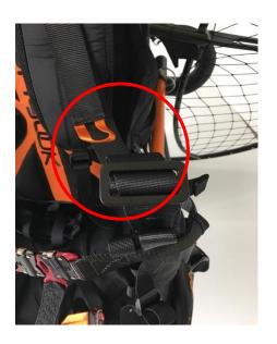
1: To adjust the straps to the right length, remove that buckle.
