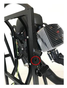
1 : Identify the drilling situated below the cage connector.
