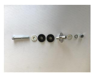
1 : Make sure that the components of the connector are set in the right order (picture).
