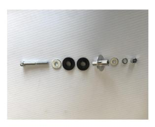
1 : Make sure that the connector components are set in the correct order (see picture).
