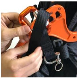
3 :Make a buckle loop with the connecting strap around the horizontal strap.
