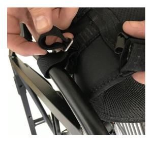
4 : Pull the strap through the second buckle, do not over tighten.
