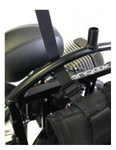
2 : Place the harness against the frame and pass the strap under the hoop.
