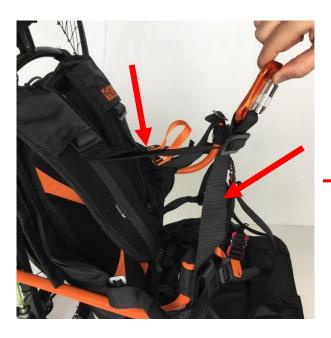
2: Adjust those two straps to calibrate the paramotor.
