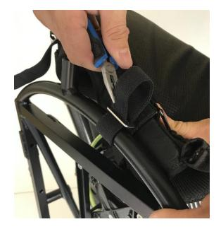
5 : Using pliers, pull the end of the strap.
