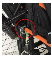
Fix the bars on the frame by means of shackles.
