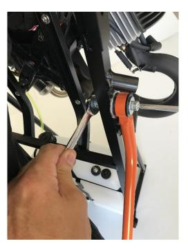
2 : Position the arm as on the picture, then attach with the spanner and the Allen key.
