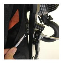
3 : Tighten with the 13 mm spanner and the 6 mm Allen key.
