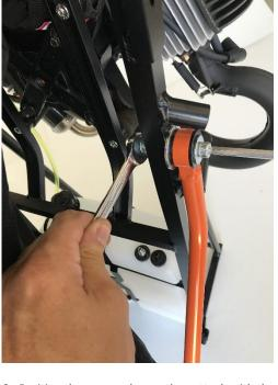
2 : Position the arm as shown, then attach with the spanner and the Allen key.
