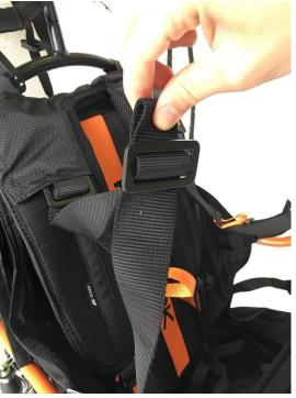
4: Replace the buckle on the mark in the opposite direction: it must be downwards.
