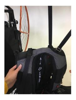
1: Put the buckle on the strap (positioned in the front) as shown. Stuff the second strap in the back of the harness or leave 5cm and cut it.
