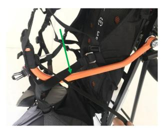
3 : Position the arm as shown. Put the end of the arm in the designed slot. Take care to pass under the strap shown by the green arrow. Position the blocking strap and add a rivet to fix the whole.
