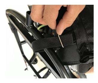
3 : Pull the strap through the first buckle. Do not over tighten.
