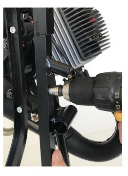
2 : Use the staged drill bit to enlarge the drilling.
