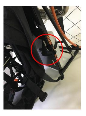
2: Unfasten the quick release buckle then attach it at the specified location.
