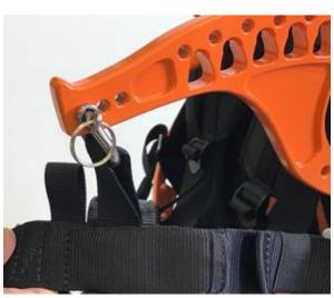
4 : Connect the previous shackle to the top of the swan neck arm (adjustment depend on the weight and comfort of the pilot).
