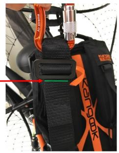
3: Once the definitive position of the buckle is chosen, mark it. Then, remove the carabiner and the buckle.
