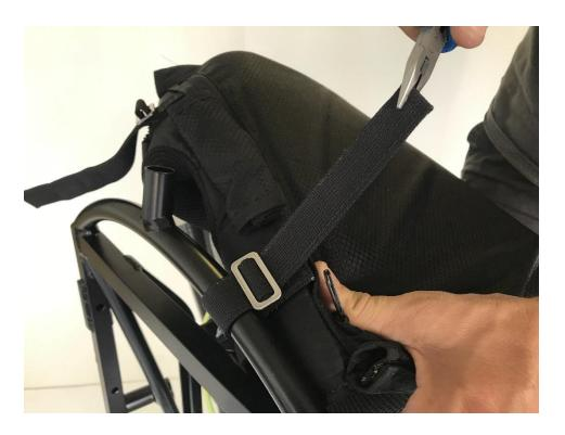
7: Tighten the strap snug to the fram and then rotate the harness forward.
